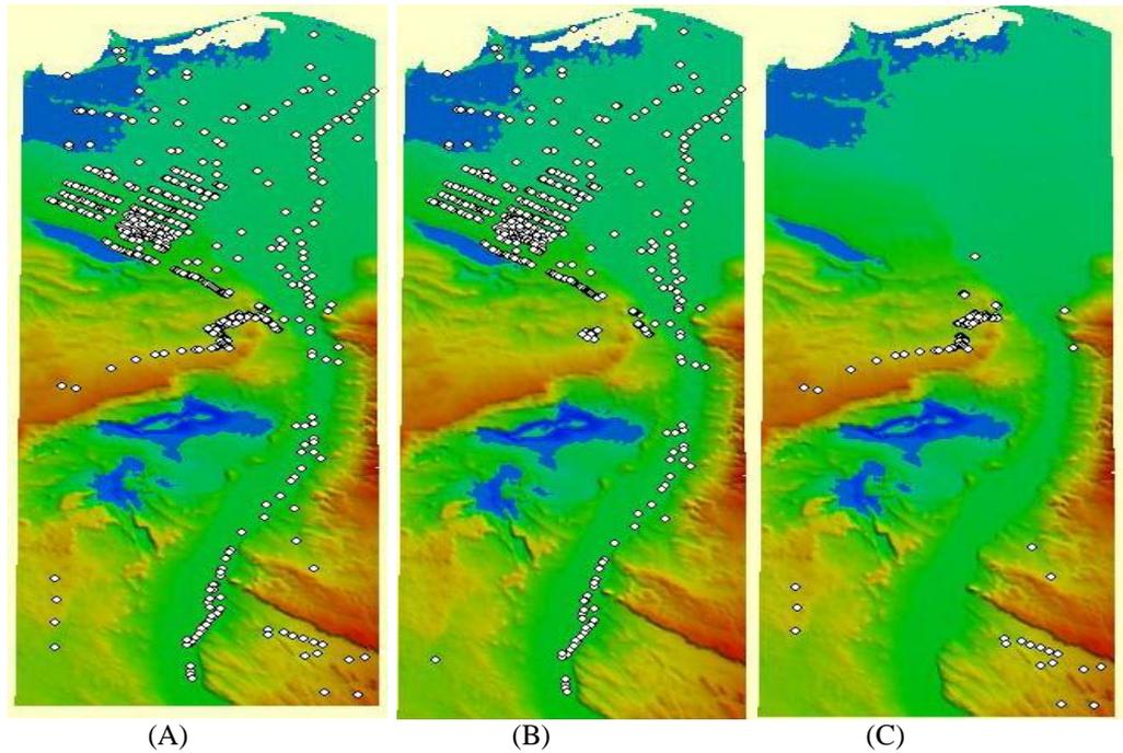
**Figure (6):** The distribution of GCPs over the flat terrain (Fig: A), steep terrain (Fig: B) and over whole terrain (Fig: C).
