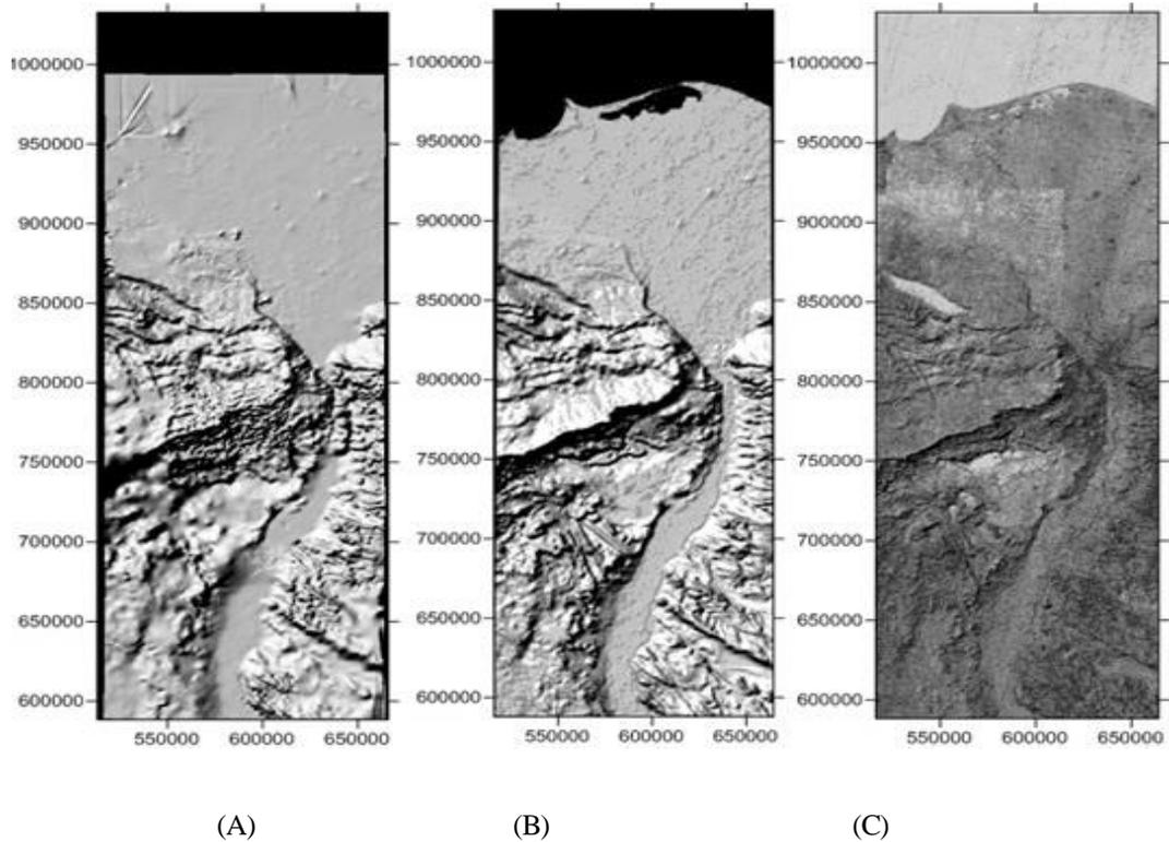
**Figure (3):** Shaded relief maps created from local DEM (A), SRTM DEM (B) and ASTER DEM (C).
