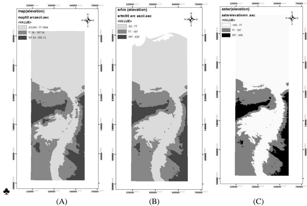
**Figure (5):** Elevation maps derived from local DEM (A), SRTM DEM (B) and ASTER DEM (C).
