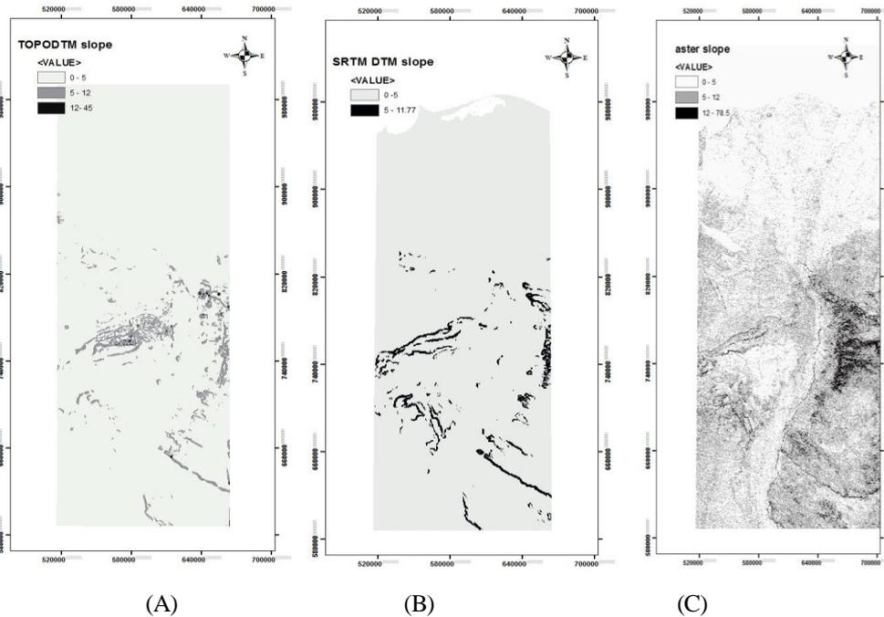
**Figure (2):** Slope maps created from the local DEM (A), SRTM DEM (B), and ASTER DEM (C)
